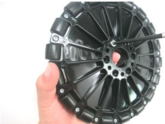
Step 8: Repeat step 7 until all six holes have been screwed into. Press a 1614ZZ shielded,  $\frac{3}{8}$ ” id ball bearing on each side of the wheel.
