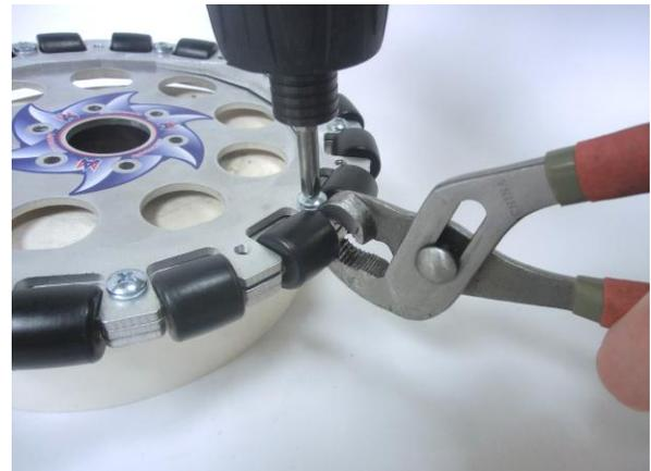
**Step 6:** Flip it over. Screw in and tighten the rest of the button head Phillip screws. Make sure it is as tight as shown below. Using a press, insert the 1/2" FR8ZZ Bearing.
