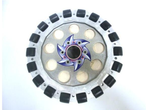
**Step 5:** Insert and tighten the 10-32 button head Phillip screws into the alternating smooth holes. If you are having trouble, use the Channellock plier to make the process run more smoothly.
