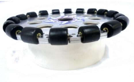
**Step 4:** Place the second outer aluminum omni ring above it, but make sure that the holes of each outer omni ring are different when on top of each other. For example, the threaded hole should be on top of the smooth hole.
