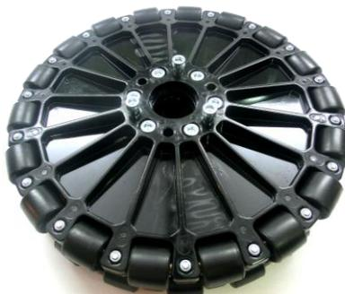
Step 4: Cover the three #10-32 x 2-1/4" SHCS with your hand and turn the wheel over. Screw in the M5 Nylock Nuts by hand.
