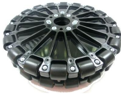
Step 6: Press in a 1/2" id flanged, shielded ball bearing to each side of the assembled dualie omni wheel.
