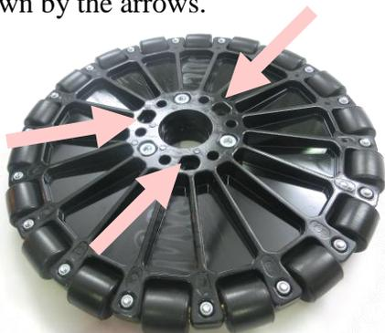
**Step 2:** Press in an R8 1/2" id bearing to the top off the first wheel, and to the bottom of the second omni wheel.
