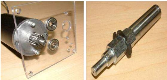
Step 4: Mount motor to Mount Plate using #10-32 screws. **DO NOT ADD Loctite or other thread locking material.** This has already been applied to the screws (excess Loctite or other thread locking material will eat away the polycarbonate). Make sure that the bearing flanges are not on the same side as the motor.
