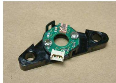
Step 3: Mount the assembly created in Step 2 to the Toughbox Mount plate, with the 2 - #10-32 screws supplied in the Package.
