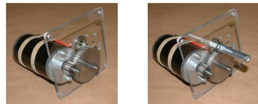
Step 6: Place the Small Hex Shaft into the bearing closest to the motor pinion. Place the Large Cluster Gear (with the smaller hex hole) onto the Small Hex Shaft. Make sure the teeth of this gear mesh well with the CIM Gear. Also, be sure to place the gear so that the small boss (raised surface) around the hex hole is facing the bearing on the Mount Plate.
