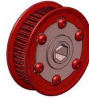
**Step 3:** Slide the pulley and hub assembly on the gearbox's hex output shaft with the Nylock nuts positioned facing out. Slide the 1/2" hex bore collar clamp (am-1238) on the gearbox hex output shaft, adjacent to the hex hub aluminum face. Place the 85 tooth belt (am-2703) around the 42 tooth pulley (am-2234).
