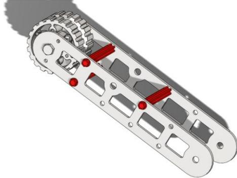
**Step 13:** Position Upper Arm assembly onto Main Body assembly so Upper Plates are outside of the Main Body plates, the 3/8" holes are aligned, and the Upper Arm is positioned as shown. Insert the 3/8" axle bolt (am-1297) into the 3/8" holes at this hinge, through these parts: Upper Plate, Outside Plate, 3/8" washer (am-1393), Pulley Wheel, brass spacer (am-2243), 3/8" washer (am-1393), Upper Plate, Inside Plate. Tighten the 3/8 nut (am-1394) on axle bolt. Back off the nut 1/2 turn.
