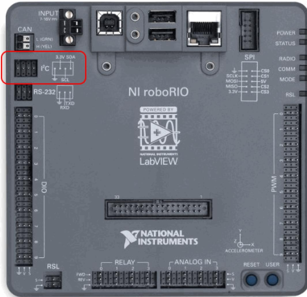
**IMPORTANT NOTE:** The left-to-right order of the RoboRIO Onboard I2C Interface Pins is different than the navX-Micro I2C pin left-to-right order.
