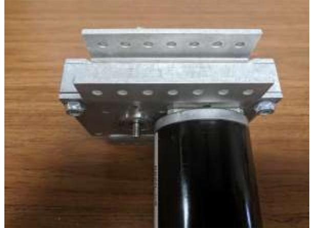
**Step 7d:** Flip the gearbox over and before installing the second spacer apply a liberal amount of grease to both gears, spin the shaft by hand to mix the grease around and into all the valleys of the gear teeth. Once greasing is complete repeat step 6d for the other spacer. Now tighten all bolts while ensuring that the output shaft still spins and that the corners of the spacers line up with the gearbox plates.
