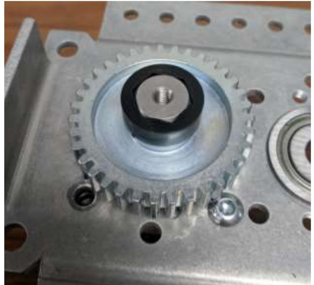
**Step 5b:** Place two #10 fender washers on the top of the shaft and secure the stack in place with a 3/8 in. long #10-32 thread patch button head cap screw.
