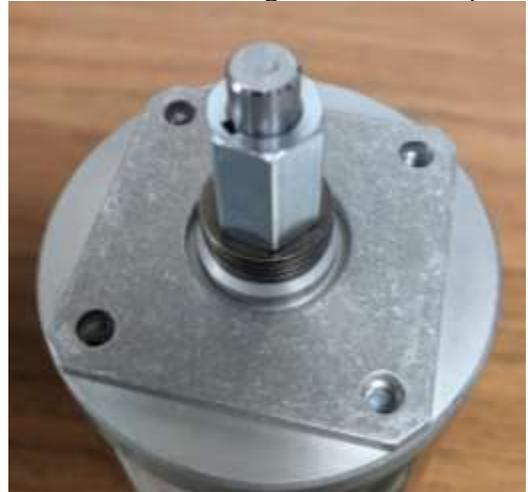
**Step 3a:** Install the 3/8 in. ID bearing in the bearing hole in the plate furthest from the bent tab. The flange of the bearing should be on the same side as the tab. Place this assembly on top of the CIM as shown.
