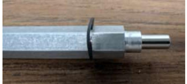
**Step 3d:** Slip the output gear onto the end of the shaft up to the snap ring. Then slip the 1/16 in. thick spacer over the 3/8 in. round portion of the shaft. Note, this spacer has a hex bore, but is being used as a round spacer in this application.
