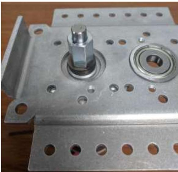
**Step 4a:** Install the 5/8 in. long thread patch button head screws into the two tapped holes of the CIM motor, then slip your pinion gear over the hex adapter. If you want the gearbox to spin faster than the CIM motor put the larger of the two gears here. If you want it to spin slower, but with more torque put the smaller gear here.
