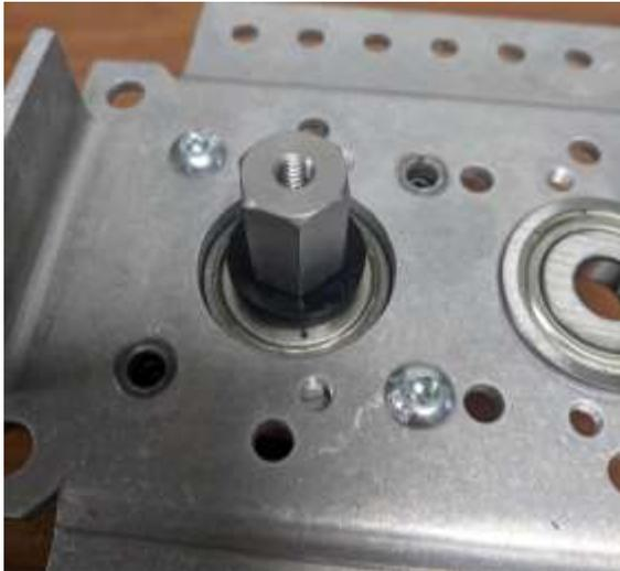
**Step 4b:** Place the pinion gear onto the 1/2 in. hex shaft then place the other 1/4 in. spacer over the gear to bring the stack flush with the top of the shaft. Again, if your shaft is different, you may need to supply your own spacers. If you want the Flyer Gearbox to spin faster than the Sport, put the larger of the two gears here. If you want it to spin slower, but with more torque put the smaller gear here.
