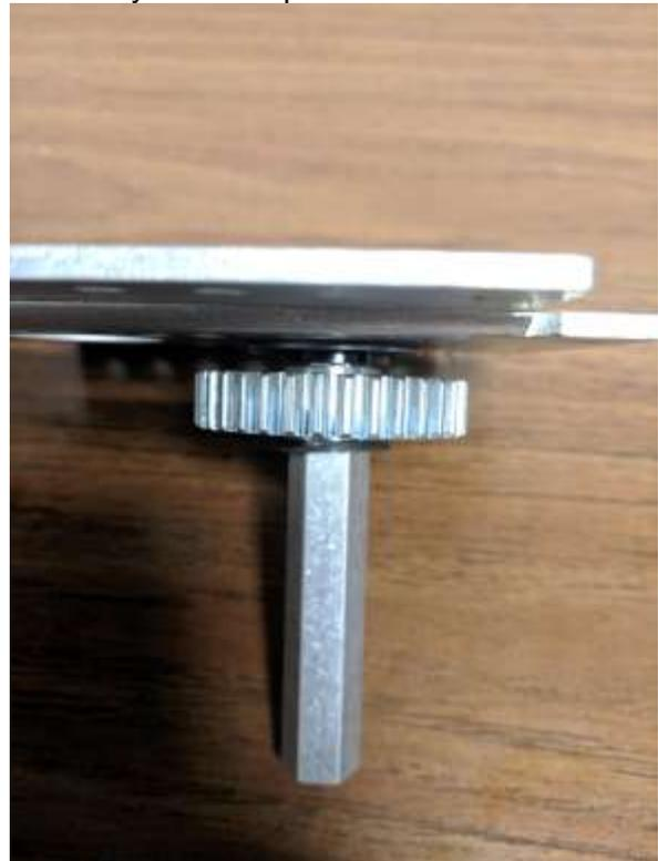
**Step 5d:** Install the 1/2 in. hex bearing with gearbox plate over the output shaft so that the tabs on both plates point at each other enclosing the gears like shown.
