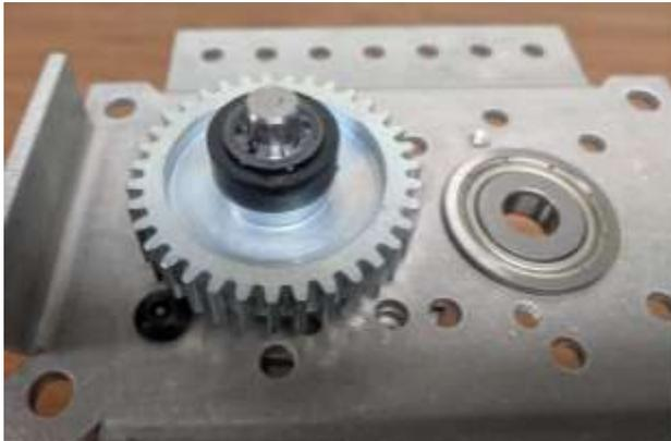
**Step 1b:** Section “b” covers preparing a 57 Sport, or similar, gearbox with a 1/2 in. hex output shaft to be the input to the Flyer. If using a Falcon 500 Please skip ahead, if using a CIM style motor go back to section “a”. Remove the two shorter screws from the face of the gearbox (we will not be using them later) and place the face mount spacer over the top with the holes aligning to the holes the screws just came out of.
