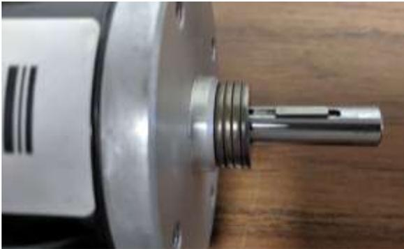
**Step 2a:** Place the 8mm key to 1/2 in. hex adapter over the shaft and place the spacer plate on the face of the motor with the holes aligned. Note: This spacer is only needed if all 4 washers were used in step 1a. It is needed to let the CIM clear the bearing in the next step.
