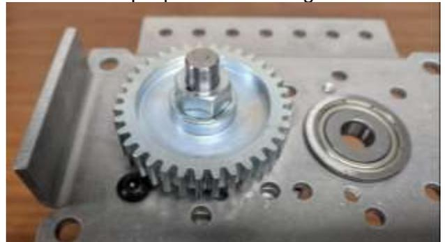
**Step 5a:** Install the 1/4 in. thick hex spacer over the gear. Then press on the 8mm retaining clip to keep all the items on the shaft. The teeth of the clip should point “up” as shown. A socket, or box end wrench is a good tool to use for this step.
