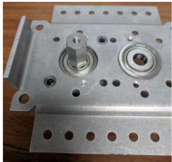
**Step 3b:** Install the two 3/4 in. long button head cap screws to hold the Sport in place, then place a 1/4 in. thick hex spacer on the output shaft. If your input is different from a sport, use your own spacers to get to 1/8 in. above the sheet metal.
