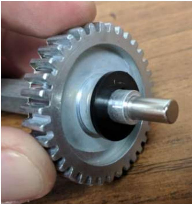
**Step 4d:** Take the output shaft assembly and insert the 3/8 in. round end of the shaft into 3/8 in. round bearing that is installed on the motor plate assembly from the previous section.
