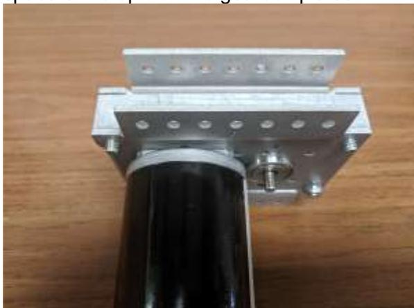
**Step 8d:** If you wish to put an encoder on the output shaft install the encoder mount pad using the two 3/8 in. long #10-32 thread patch button head cap screws. The screws thread into the gearbox plate for easy installation and removal without disassembly of the gearbox
