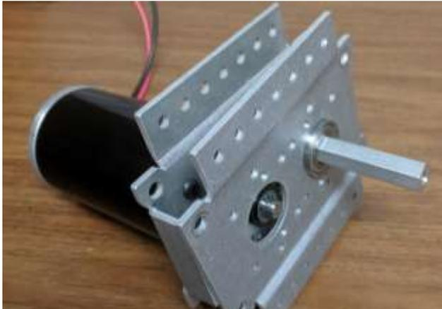
**Step 6d:** Place the extrusion spacer in the gap on one side of the gearbox. Feed 1/4-20 button head cap screws through the corner holes in the gearbox plate, the holes in the spacer and out the holes in the opposite gearbox plate. Secure in with locknuts. Note, do not tighten down the nuts all the way yet.
